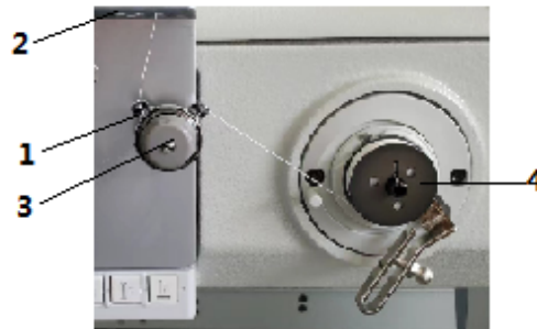
Fig. 17: Winding the hook thread (2)
