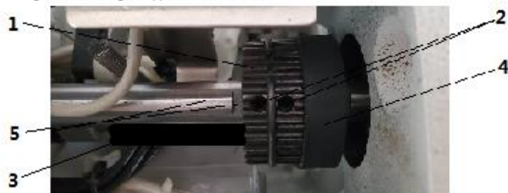
Fig. 44: Positioning the upper toothed belt wheel
