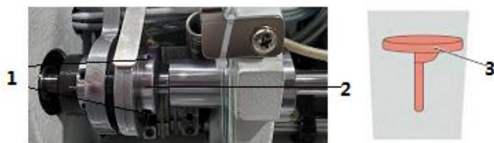
(1) - Threaded pins (2) - Pusher eccentric (3) - Stitch regulator
