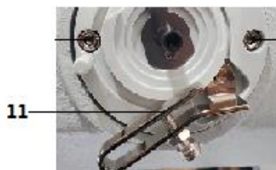
Fig. 82: Adjusting the winder (3)
