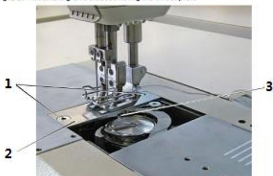
Fig. 36: Assembling and disassembling the throat plate
