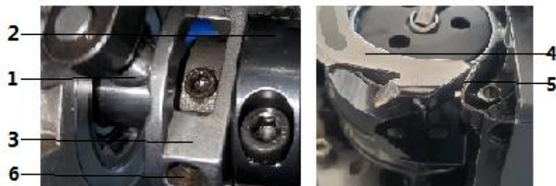
Fig. 90: Adjusting point in time for cutting
