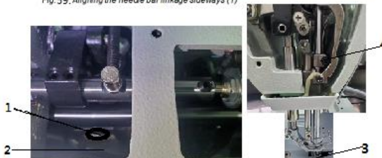
Fig. 59: Aligning the needle bar linkage sideways (1)
