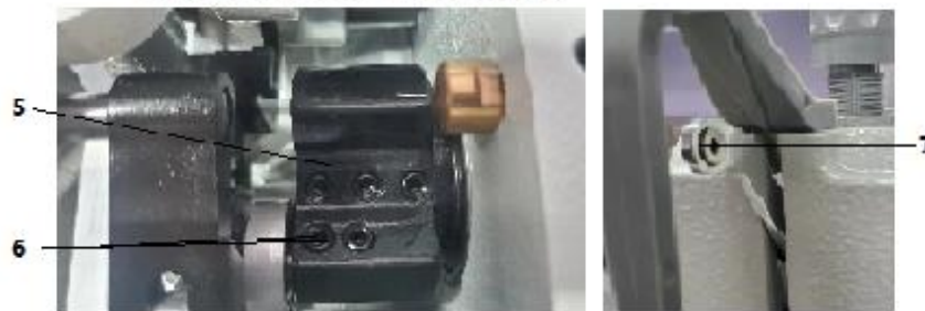
Fig 60: Aligning the needle bar linkage sideways (2)
