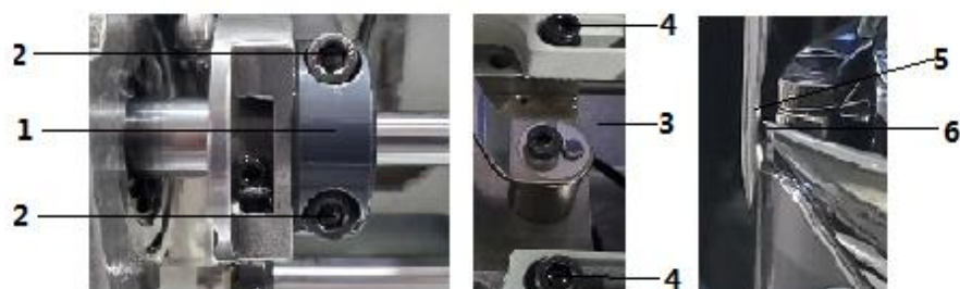
Fig.62: Adjusting the hook side clearance
