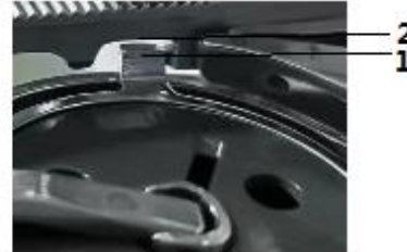
(2) - Slot in the throat plate
