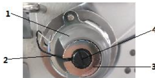
(1) - Stop collar (2) - Spring (3) - Tension disk (4) - Screw
