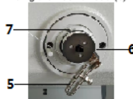
Fig. 18: Winding the hook thread (3)
