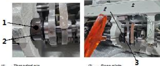
Fig. 56: Adjusting the compensating weight
