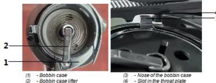
Fig 67: Adjusting the bobbin case lifter
