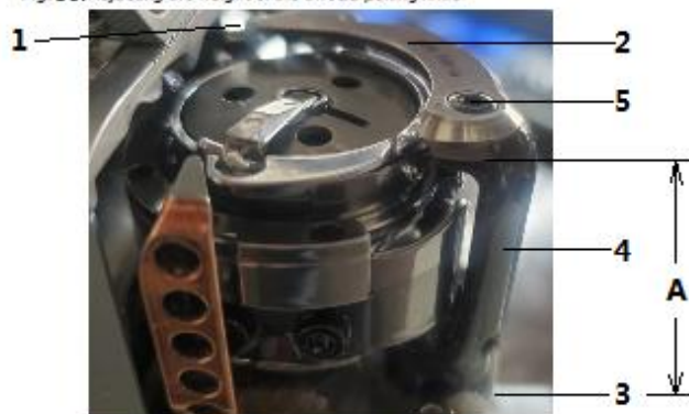
Fig. 86: Adjusting the height of the thread-pulling knife
