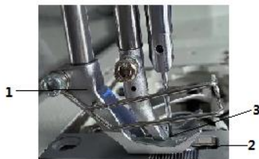
(1) - Walking foot (2) - Feed dog (3) - Needle tip
