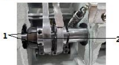
Fig. 57: Adjusting the stroke movement
