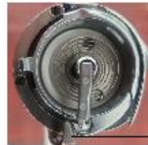
(5) - Screw (6) - Bobbin case lifter
