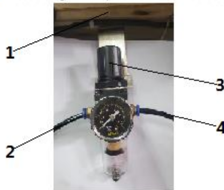
Fig. 4: Assembling the compressed air maintenance unit
