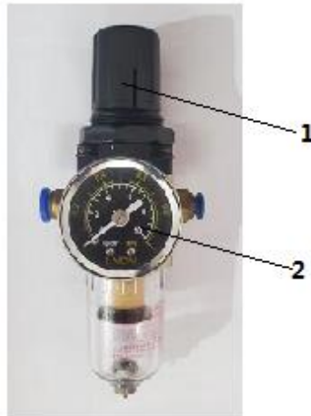
Fig. 5: Setting the operating pressure
