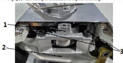
Fig. 37: Assembling and disassembling the feed dog
