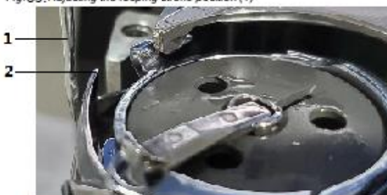
Fig.63: Adjusting the looping stroke position (1)
