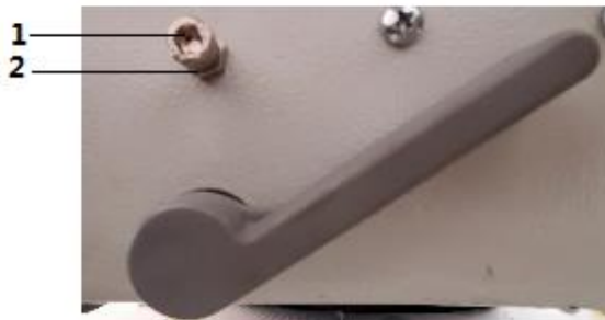
Fig. 76: Adjusting the sewing foot lifting height
